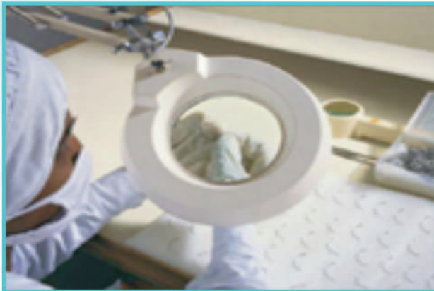
Needle inspection under illuminated magnifying glass Checking minute defects
